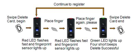
**Note:** If the fingerprint has not been deleted in the unit, the red LED will flash twice and two long beeps will occur. Therefore, try again.
