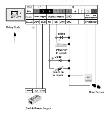
T5Pro/T5: Connect to controller as a access control reader:
