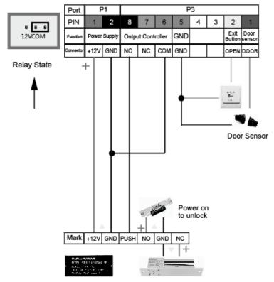
Access Control Power Supply Power off to unlock
