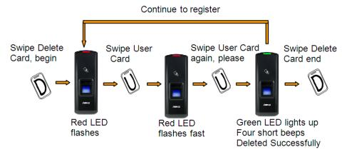
**Note:** If the fingerprint has not been deleted from the unit, the red LED will flash twice and two long beeps will occur. Therefore, try again.
